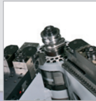
New quick die change equipment for combined rotary-draw and free- form bending
