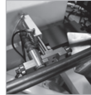
Weld seam detection
