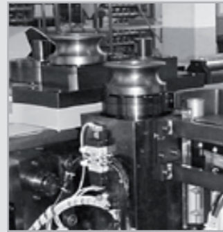
RRB42 - Pitch- and Ø-adjustment
