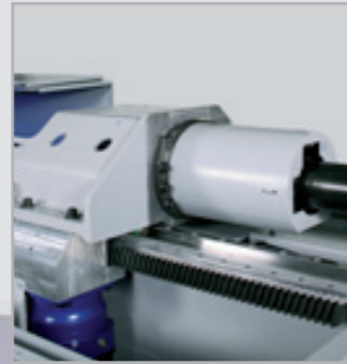
Tube positioning with boost pressure function of advance feed unit
