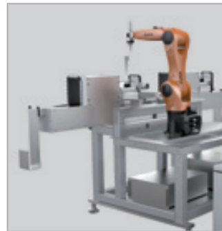
Shuttle system for workpiece feeding
